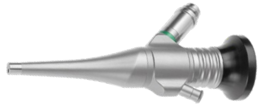
Otoscope, 5 Charr., Ø 4mm, 65mm working length
