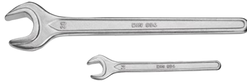
Schraubenschlüssel Set (SW30/SW17)
